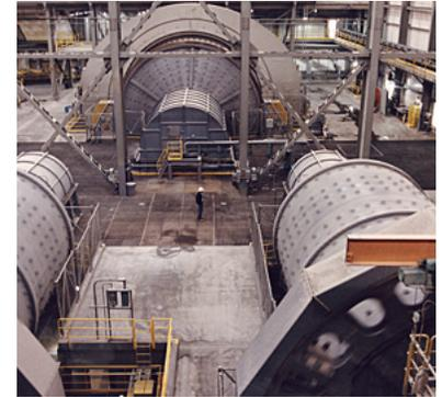
Pictured: mills used to process ore shown in the concentrator plant
